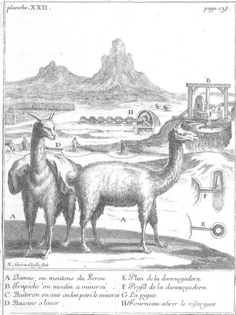
Figure 4. Trapiche according to Frézier, 1732. B = Trapiche mill to crush minerals. D = Ponds to wash the amalgam. H = Furnaces to extract the mercury.
