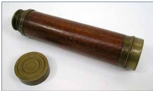
Fig. 9 (Top and below) Telescope, with main wooden tube and three brass-plated drawtubes, signed 'W. Eastland'. Achromatic triplet. F_{\text{objective}} = 380 \text{ mm} ( \approx 15 \text{ inch} ), \varnothing = 29 \text{ mm} . Aperture ratio \approx f/13 . The construction of the used brass-plated drawtubes was patented in 1782 by the London instrument maker Joshua Lover Martin, the son of the well-known London instrument maker Benjamin Martin. As William Eastland died in The Hague in 1787, this telescope seems to have been made there between 1782 and 1787. However, the clamp type cover depicted emerges around 1800. Therefore the telescope was probably produced by Eastland's companion Jonas Regenboog, who used the firm name "W. Eastland & Co" until his death in 1839. Hypothetically Eastland's former apprentice William II Eastland would also qualify as the maker of this telescope, but as far as is known he was imprisoned in 1774 and was no longer active as an optician after that time. This instrument was discovered in a Dutch antiques shop in 2011 and was purchased by the late Dick Regenboog (1941-2013), descendant of Eastland's Dutch associate Jonas Regenboog.
