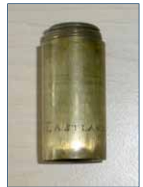
Fig. 9 (Top and below) Telescope, with main wooden tube and three brass-plated drawtubes, signed 'W. Eastland'. Achromatic triplet. F_{\text{objective}} = 380 \text{ mm} ( \approx 15 \text{ inch} ), \varnothing = 29 \text{ mm} . Aperture ratio \approx f/13 . The construction of the used brass-plated drawtubes was patented in 1782 by the London instrument maker Joshua Lover Martin, the son of the well-known London instrument maker Benjamin Martin. As William Eastland died in The Hague in 1787, this telescope seems to have been made there between 1782 and 1787. However, the clamp type cover depicted emerges around 1800. Therefore the telescope was probably produced by Eastland's companion Jonas Regenboog, who used the firm name "W. Eastland & Co" until his death in 1839. Hypothetically Eastland's former apprentice William II Eastland would also qualify as the maker of this telescope, but as far as is known he was imprisoned in 1774 and was no longer active as an optician after that time. This instrument was discovered in a Dutch antiques shop in 2011 and was purchased by the late Dick Regenboog (1941-2013), descendant of Eastland's Dutch associate Jonas Regenboog.
