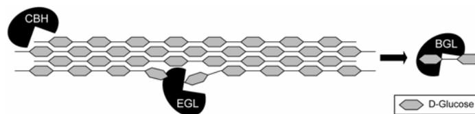
**Figure 1:** Schematic presentation of cellulose, its degradation and release of D-glucose. Reprinted from [3] with permission from the publisher (Copyright remains with the original publisher).
